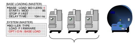
Enable the base load feature by setting:
